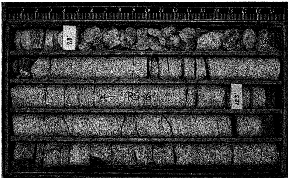
Boring B2-B – Station 19+40 @ 15' Right – Box 1 of 3
