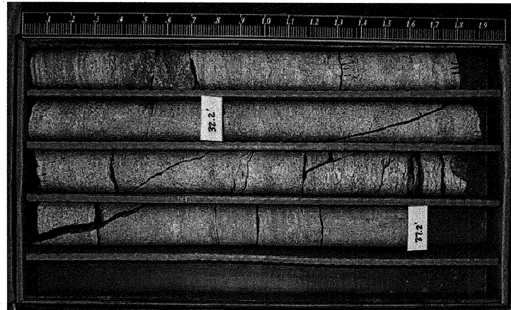
Boring B2-A – Station 19+71 @ 15' Left – Box 3 of 3
