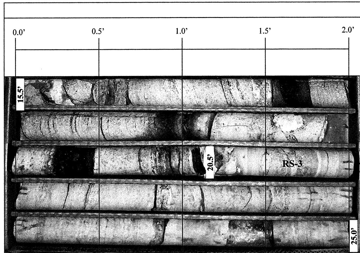
Boring B2A, Box 1 of 2, 15.5 feet to 25.0 feet.
