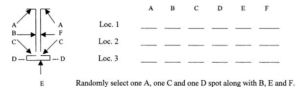
**B.** Two random adhesion tests per span are conducted on interior surfaces after the paint has been properly cured, and will be touched up by the Contractor.
