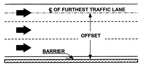
Based on the clear distance, offset, design speed and pavement type, choose an unanchored PCB, anchored PCB or an Oregon barrier from the table below:
