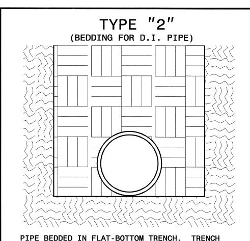
PIPE BEDDED IN FLAT-BOTTOM TRENCH. TRENCH BACKFILLED IN LOOSE 6" LAYERS COMPACTED TO TOP OF TRENCH USING LOCAL EXCAVATED MATERIAL, IF APPROVED BY THE ENGINEER, OR SELECT MATERIAL. ALL MATERIAL SHALL BE FREE OF ROCKS, FOREIGN MATERIAL, AND FROZEN EARTH. COMPACTION SHALL BE TO APPROX. 95% DENSITY IN ACCORDANCE WITH AASHTO T-99 AS MODIFIED BY THE DEPARTMENT OF TRANSPORTATION.
