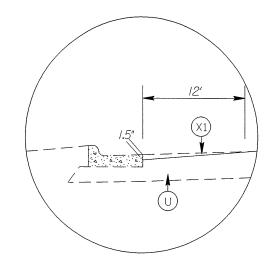
DETAIL FOR PROFILE MILLING (O"TO 1.5")
