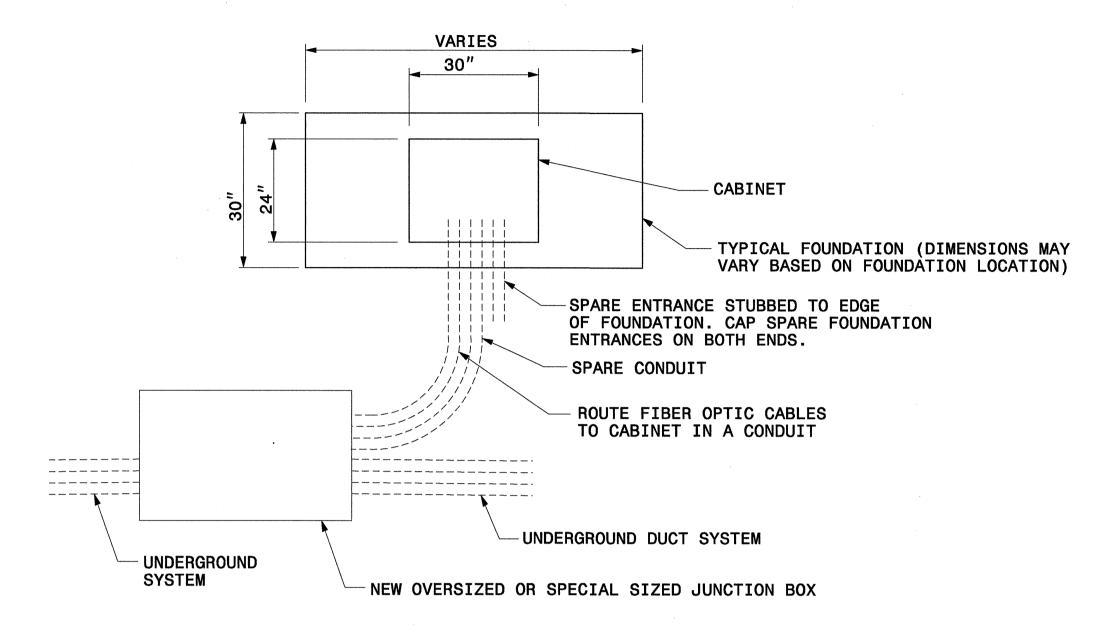
ROUTING OF CABLE TO BASE MOUNT CABINET (PLAN)
