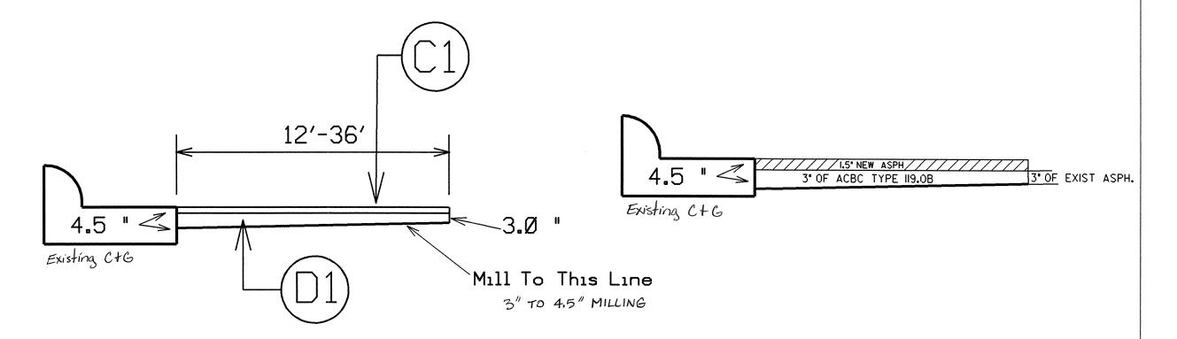
Mill Left Turn Lane And Both Thru Lanes For A Distance Of 150'
