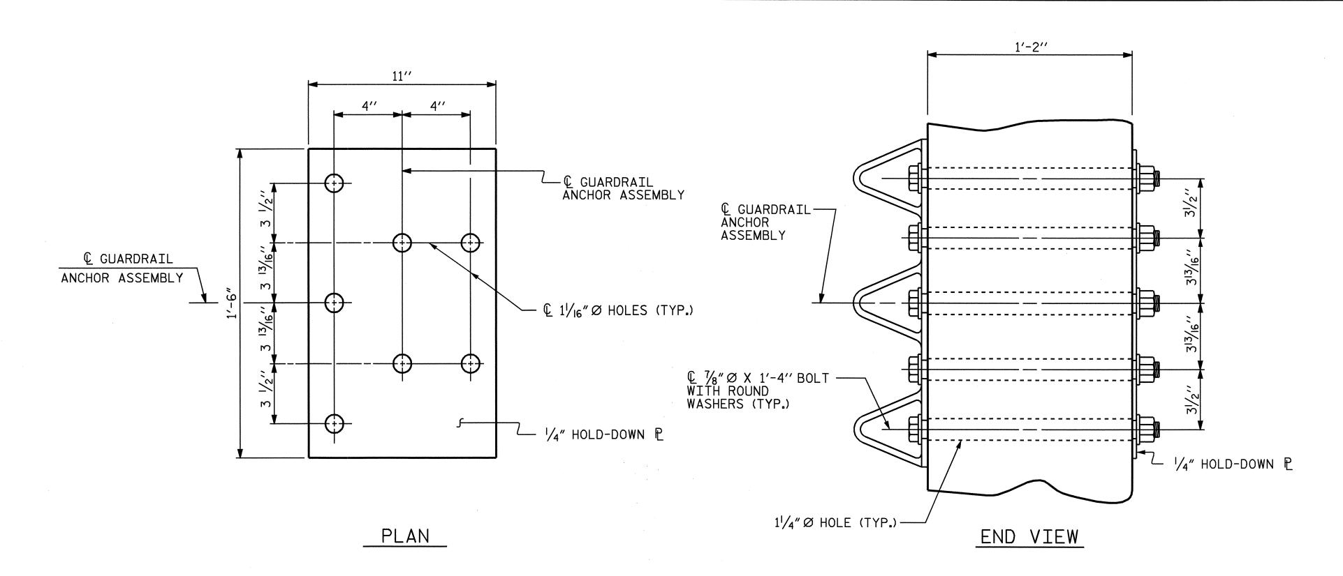
GUARDRAIL ANCHOR ASSEMBLY DETAILS
