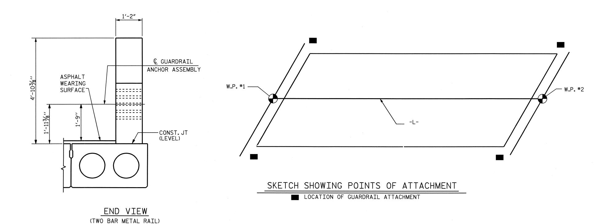
LOCATION OF GUARDRAIL ANCHOR AT END POST
