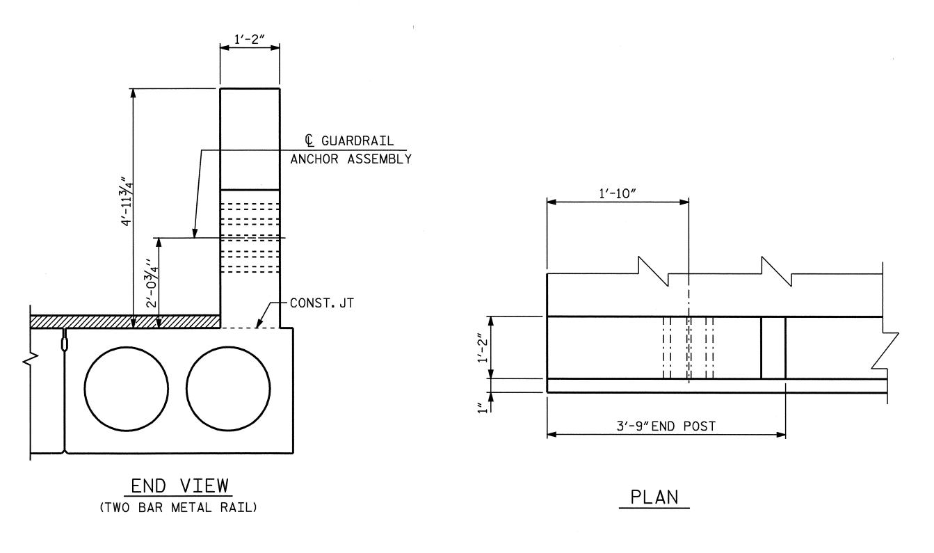
LOCATION OF GUARDRAIL ANCHOR AT END POST
