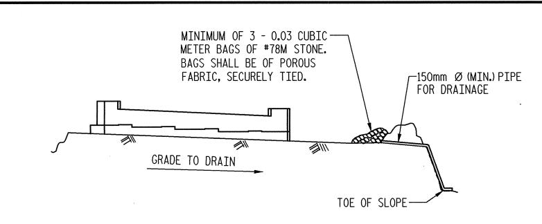
BAGGED STONE AND PIPE SHALL BE PLACED IMMEDIATELY AFTER COMPLETION OF END BENT EXCAVATION. PIPE MAY BE EITHER CONCRETE, CORRUGATED STEEL, CORRUGATED ALUMINUM ALLOY, OR CORRUGATED PLASTIC. PERFORATED PIPE WILL NOT BE ALLOWED.
