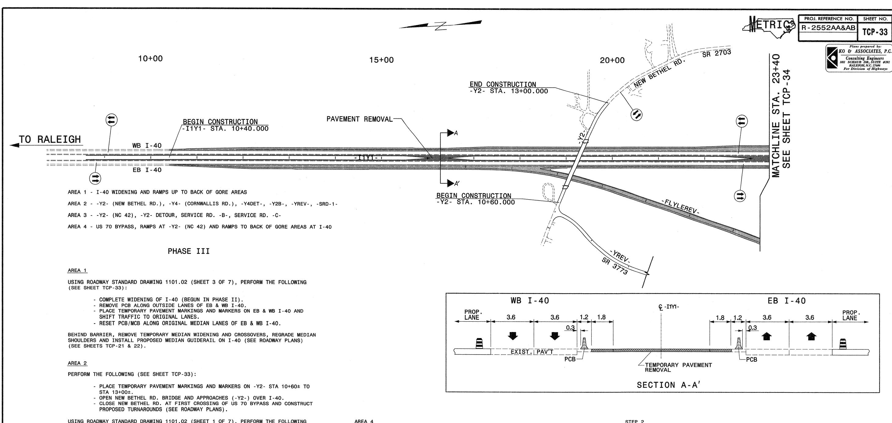
USING ROADWAY STANDARD DRAWING 1101.02 (SHEET 1 OF 7), PERFORM THE FOLLOWING (SEE SHEETS TCP-35):
