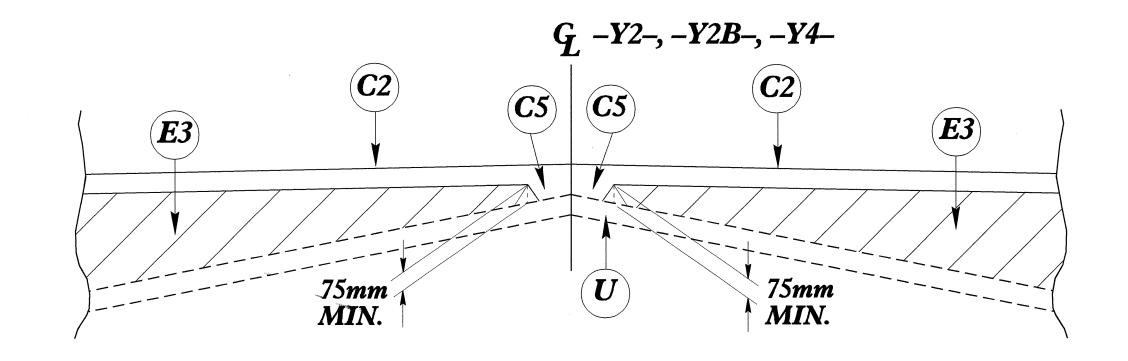
DETAIL SHOWING METHOD OF WEDGING NO. 1 USE IN CONJUNCTION WITH TYPICAL SECTIONS NO. 5 & NO. 9
