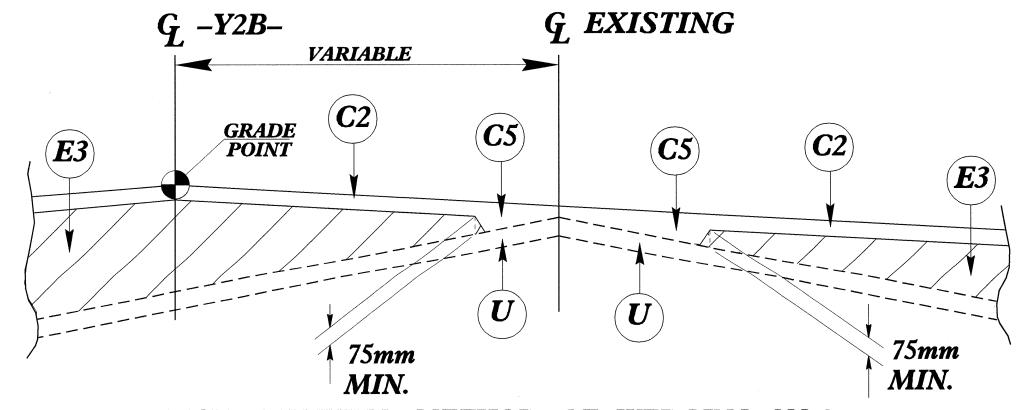
DETAIL SHOWING METHOD OF WEDGING NO.2 USE IN CONJUNCTION WITH TYPICAL SECTION NO. 5
