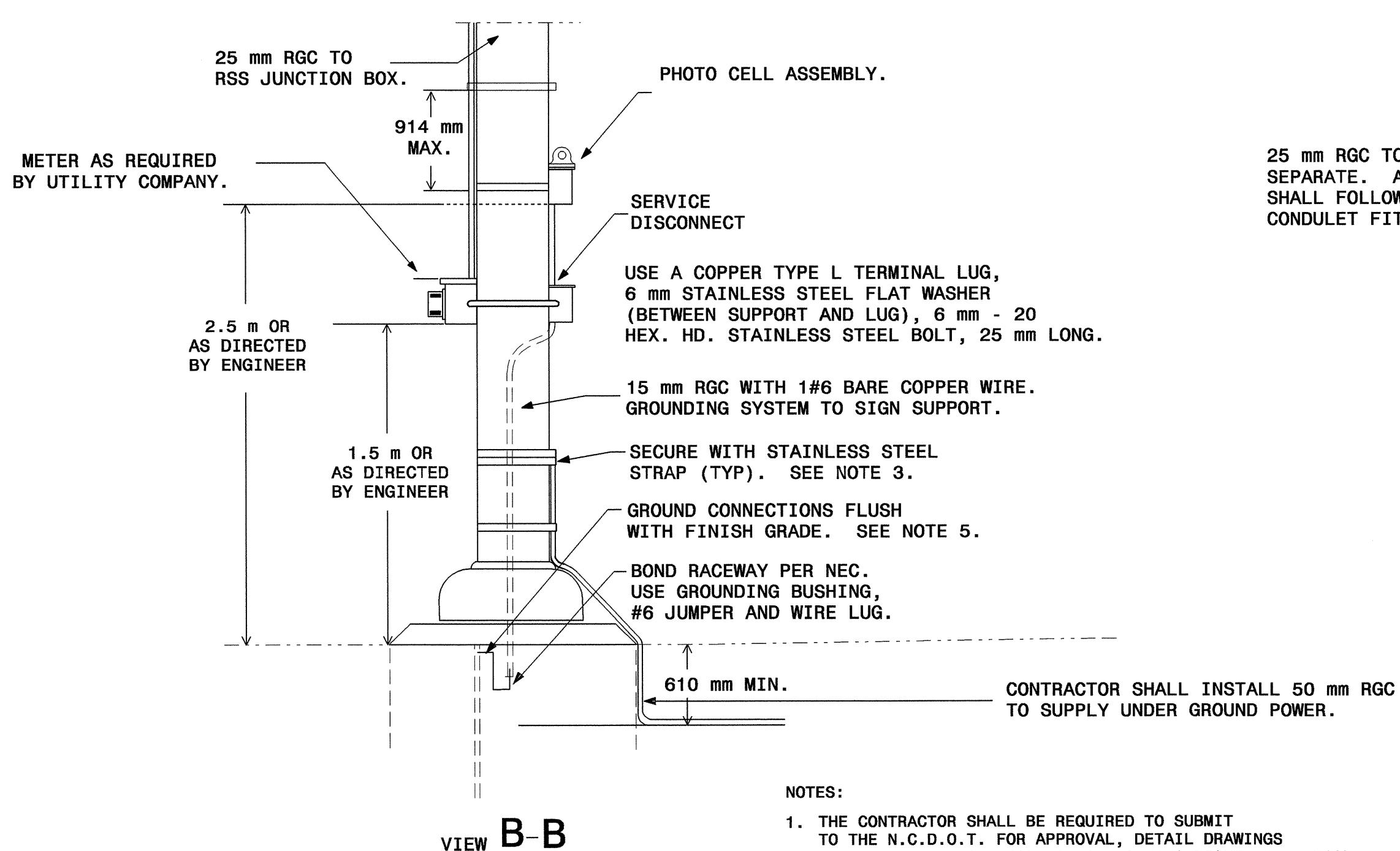
25 mm RGC TO RSS JUNCTION BOX WHERE CIRCUITS SEPARATE. ALL CONDUIT INSTALLED ON STRUCTURE SHALL FOLLOW STRUCTURAL MEMBERS USING 90 DEGREE CONDULET FITTINGS AT EACH 90 DEGREE DIRECTIONAL CHANGE.
