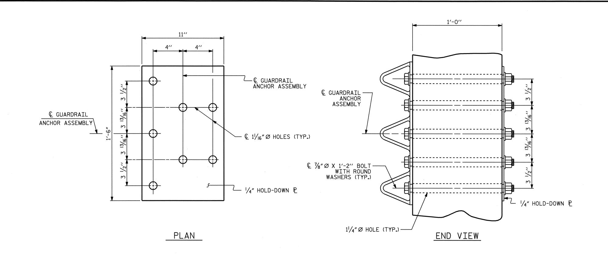
GUARDRAIL ANCHOR ASSEMBLY DETAILS
