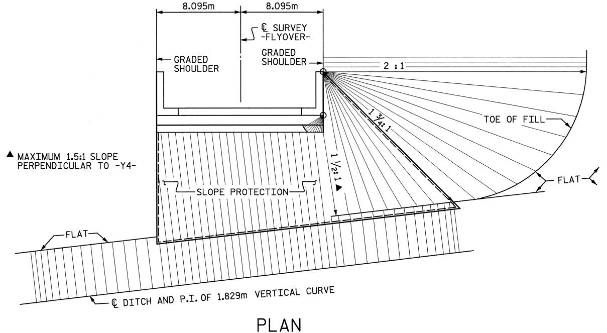
END BENT 1 SHOWN, END BENT 2 SIMILAR BY ROTATION
