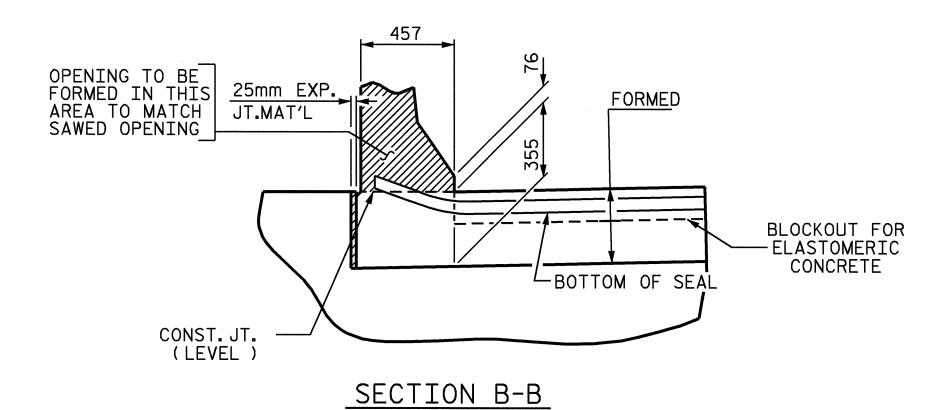
JOINT SEAL DETAILS @ END BENT
