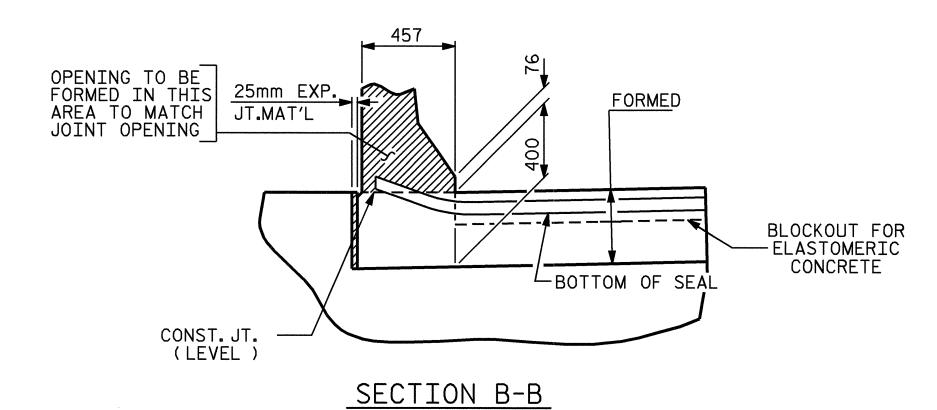
JOINT SEAL DETAILS @ END BENT (FOR BARRIER RAIL)
