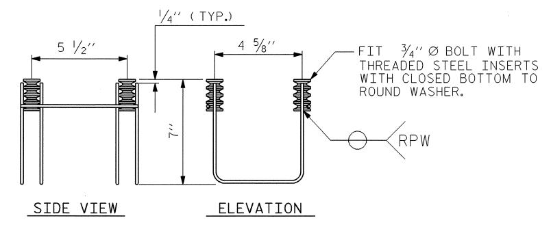
MINIMUM LENGTH OF THREADS IN INSERT (FERRULE):  $1\frac{3}{4}$
