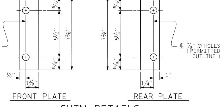
SHIMS MAY BE CUT ALONG PERMITTED CUTLINE OR SLOTTED TO EDGE OF PLATE TO FACILITATE PLACEMENT.
