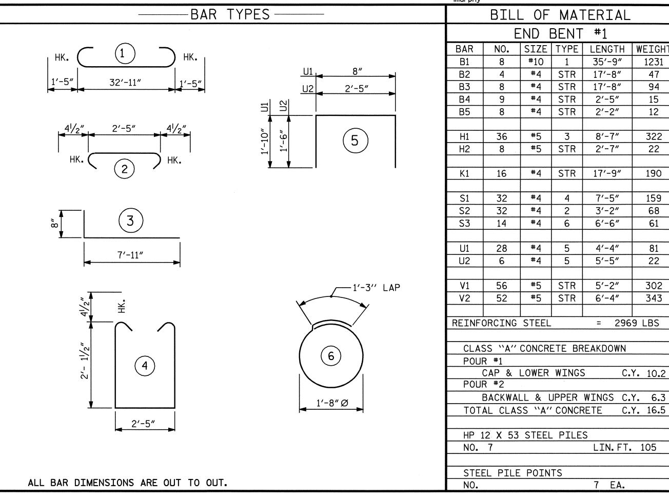
PROJECT NO. ASHE 19+05.00 -L-STATION: SHEET 3 OF 3 STATE OF NORTH CAROLINA DEPARTMENT OF TRANSPORTATION SUBSTRUCTURE END BENT #1
