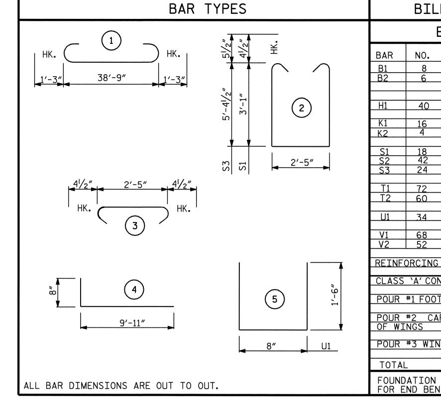
BILL OF MATERIAL END BENT #2 TYPE | LENGTH | WEIGHT 5 4 9'-9" STR 20'-8" 4 STR 2'-7" 9'-0" 60 STR 6'-3" 563 34 5 3′-8″ 52 5 STR 8'-1" REINFORCING STEEL CLASS 'A' CONCRETE POUR #1 FOOTINGS C.Y. POUR #2 CAP, LOWER PART OF WINGS C.Y. 16.0 POUR #3 WINGS & BACKWALL C.Y. C.Y. 39.8 FOUNDATION EXCAVATION FOR END BENT #2 LUMP SUM
