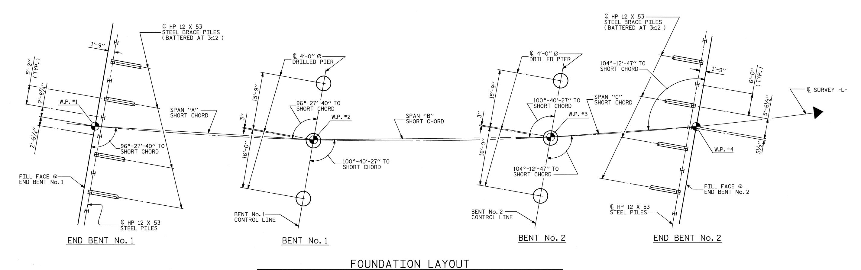
(DIMENSIONS LOCATING PILES ARE TO THE CENTERLINE OF THE PILE AT THE BOTTOM OF THE CAP
