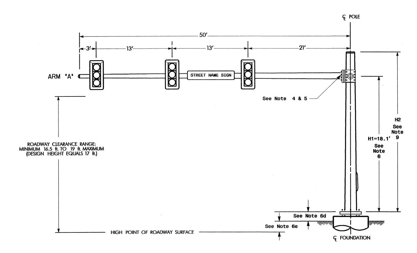
Design Loading for METAL POLE NO. 7, MAST ARM A
