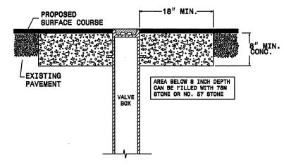
USE RAPID SET GROUT, MORTAR, OR CONCRETE CLASS B CONCRETE MAY BE USED WHEN ADJUSTMENTS ARE NOT IN THE TRAVEL LANE.
