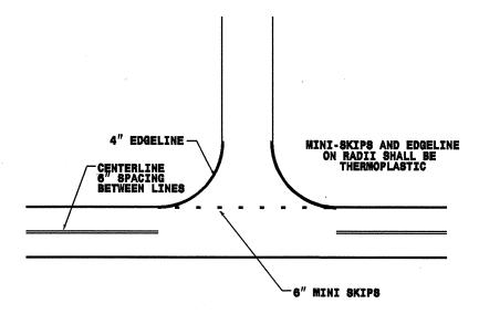
NOTE: MINI SKIPS SHALL BE PLACED ON A 10' CYCLE, CONTAINING AN 8' AND 2' SKIP, THE WIDTH OF THE SKIP SHALL BE 6".
