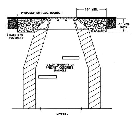
1. MORTAR SHALL BE MIXED TO NCDOT SPECIFICATIONS.
