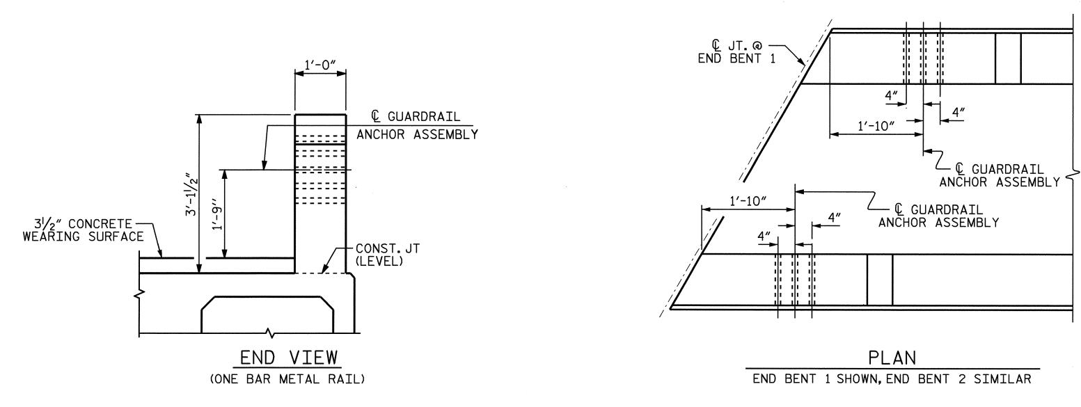
LOCATION OF GUARDRAIL ANCHOR AT END POST
