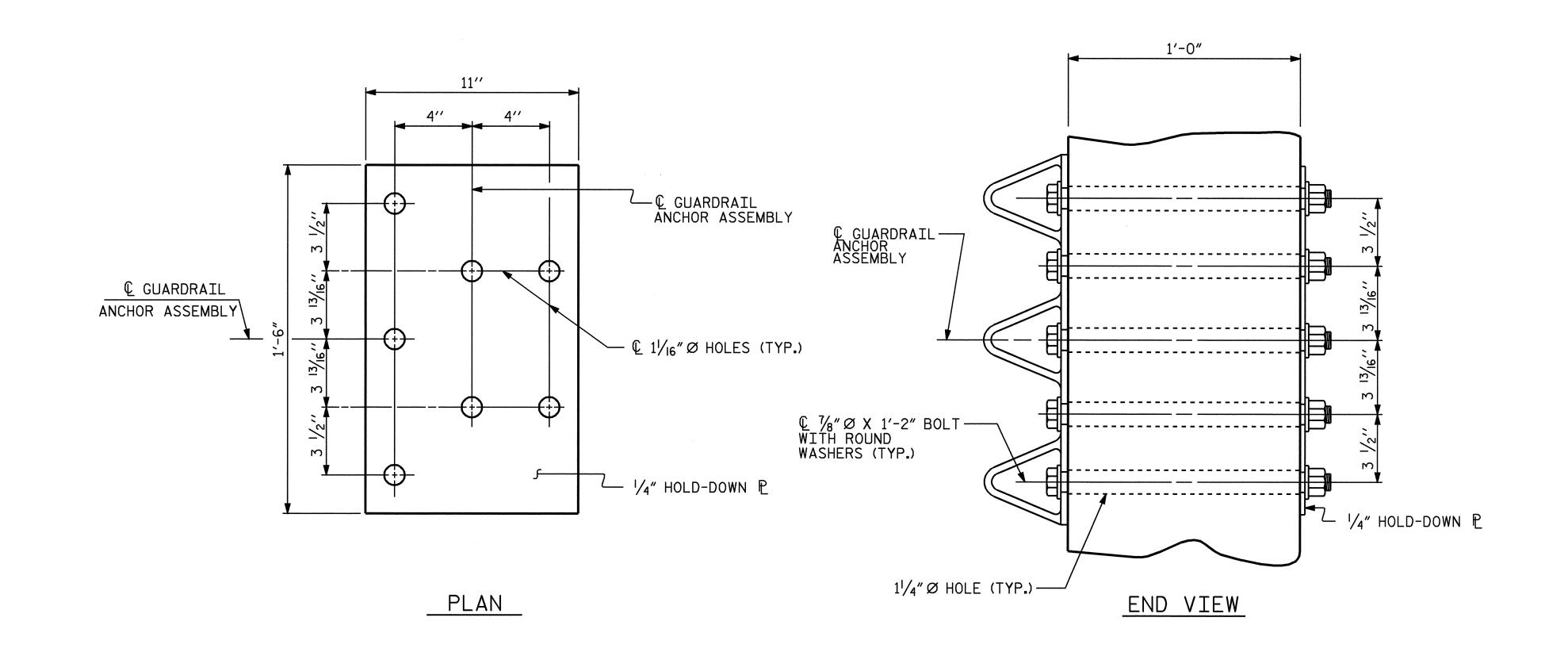
GUARDRAIL ANCHOR ASSEMBLY DETAILS
