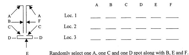
**B.** Two random adhesion tests per span are conducted on interior surfaces after the properly cured.
