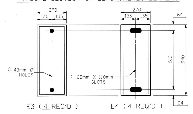
PLAN VIEW OF ELASTOMERIC BEARING
