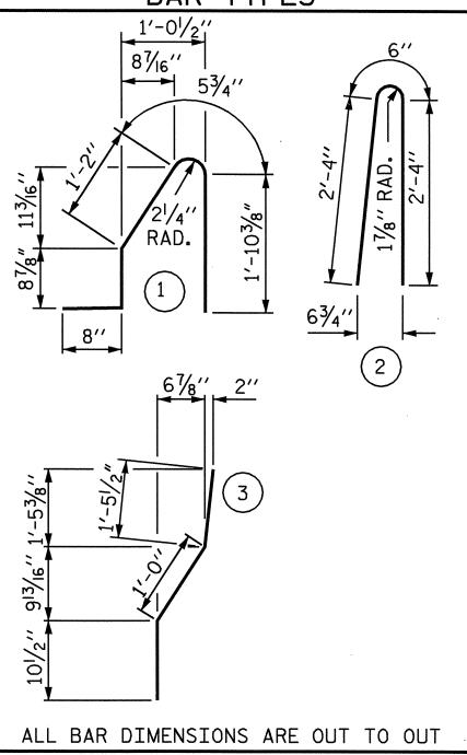
BILL OF MATERIAL FOR CONCRETE BARRIER RAIL ONLY BAR NO. SIZE TYPE LENGTH WEIGHT 260 #5 1 1,333 4'-11" **₩** S1 5'-2'' 260 #5 2 1,401 12 #5 3 \*S3 3'-4'' 42 **\***S4 12 **\***5 STR 3'-2'' 40
