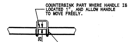
PART SECTION THRU COVER SHOWING HANDLE
