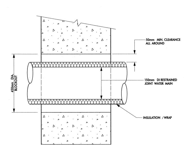
SECTION THRU CONTINUOUS DIAPHRAGM
