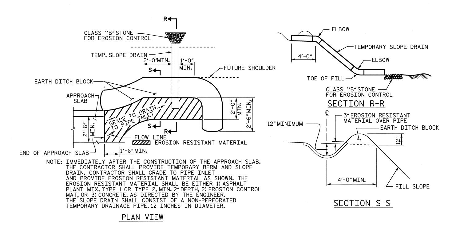
TEMPORARY BERM AND SLOPE DRAIN DETAILS
