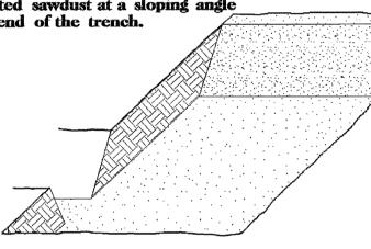
4. Place a single layer of plants against the sloping end so that the root collar is at ground level.
