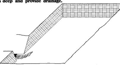
3. Backfill the trench with 2 inches we rotted sawdust. Place a 2 inch layer well rotted sawdust at a sloping angle
