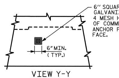
6" SQUARE ALUMINUM OR GALVANIZED STEEL WIRE 4 MESH HARDWARE CLOTH OF COMMERCIAL QUALITY. ANCHOR FIRMLY TO FILL
