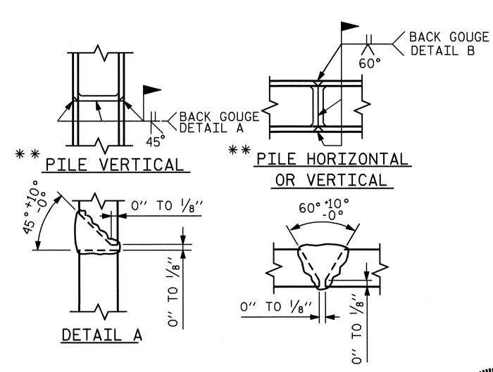
DETAIL B POSITION OF PILE DURING WELDING.
