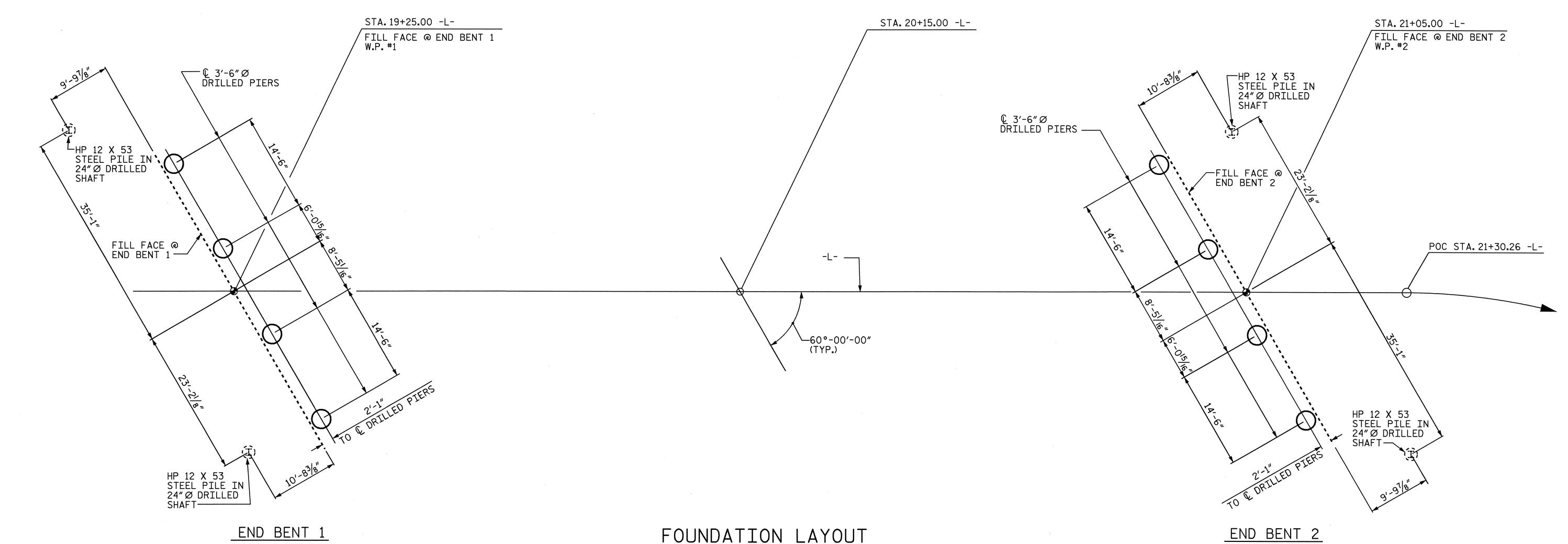
DIMEMSIONS LOCATING PILES ARE TO THE PILE CENTERLINE.
